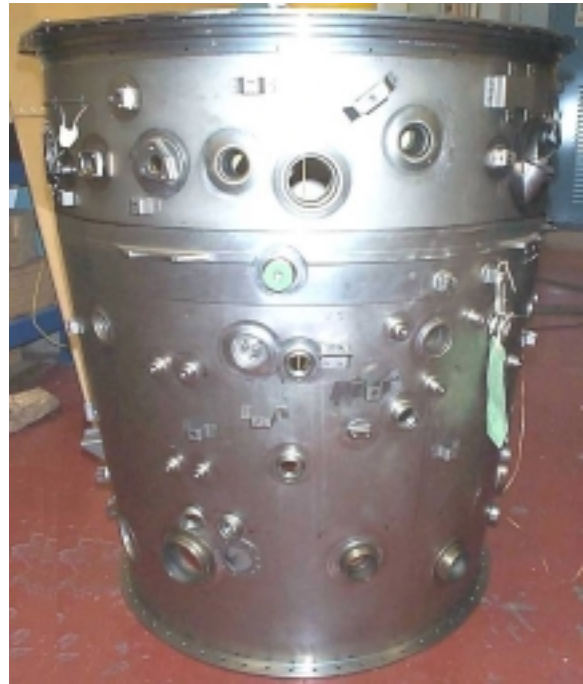
Figure 2: Investigated bypass duct (Rolls-Royce plc.)
