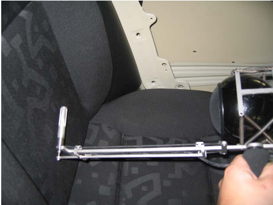
Figure 8: Measurement with Microflown device inside the body in white
