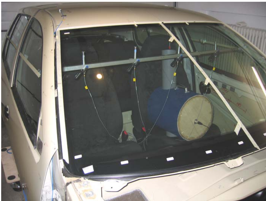
Figure 4: Sound source inside body in white with microphone array
