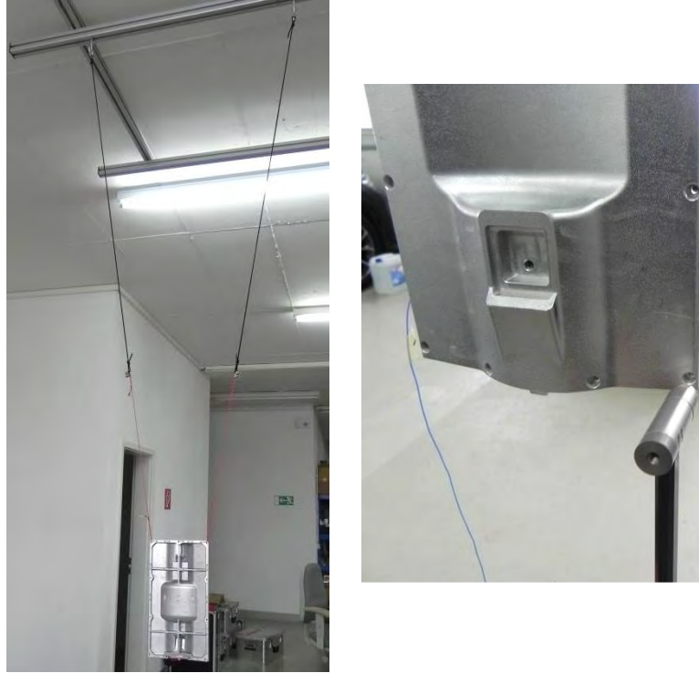
Figure 2: Survey of classical hammer test (reference test)
