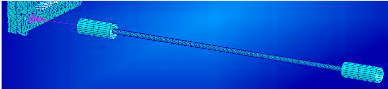
Figure 15: FE model of impedance head/stinger assembly
